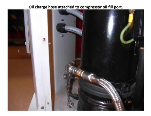
7. Slowly attach the other side of the oil flex line to the oil vessel and transfer the oil. You will know that the transfer is complete when you hear the bubbling sound of helium passing through oil tank (depend on pressure difference this can take 15-60 seconds)
