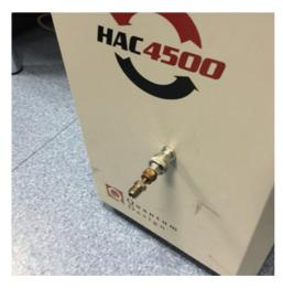
3. In case of air-cooled compressor, the oil will be charged to capsule located in outdoor unit. In case of water-cooled compressor, the oil will be charged to capsule located in indoor unit. Bring the oil fill tanks and the helium cylinder to the compressor unit to be filled. Let the oil fill tanks stay in upright position for about 15min at least before continuing!
