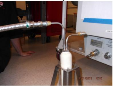
6. Attach the oil flex (short) line to compressor oil fill port.
